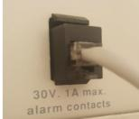
When looking at your connections, you are looking to find the **normally closed** contacts. These are the contacts that are connected together when the machine is not in alarm. This is important for robustness – anything that breaks the loop of wire will end up triggering an alarm – be it an actual alarm, or, if the wire becomes disconnected.
